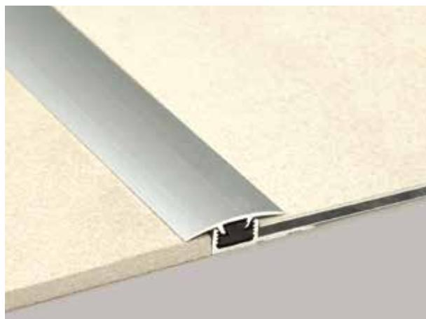
Patented coplanar joint profile. The innovative, ingenious clip system in Resinil (thermoplastic synthetic resin) allows, by simple rotation, to compensate level differences of up to 1.5 mm. The system can also join floors with thicknesses varying from 4 to 6 mm. It additionally acts as a movement joint profile, since the internal cavity allows the underlying flooring to move up to  $\pm$  2 mm.
